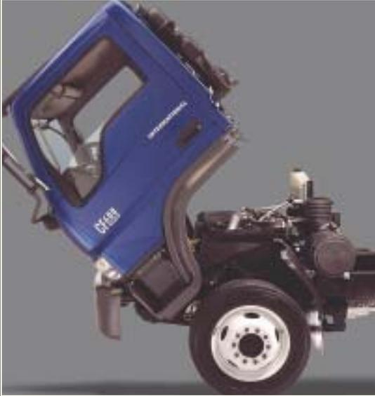
**The International® CF Series offers easy, efficient daily maintenance – with a full-tilt cab and easily accessible service points. The CF Series powertrain, chassis and cab offer streamlined maintenance intervals for cost-effective repairs and maximum uptime.**
